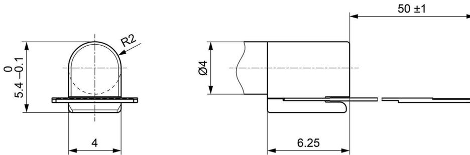
Figure 2 Dimensional Drawing [mm] – ENX 4 MAG
