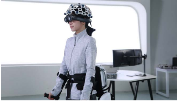
Fourier's exoskeleton, ExoMotus™ X2 combining EEG controlling module. Powerful Actuating Unit – a high-performance motor and gearhead to provide a stronger torque output © Fourier Intelligence
