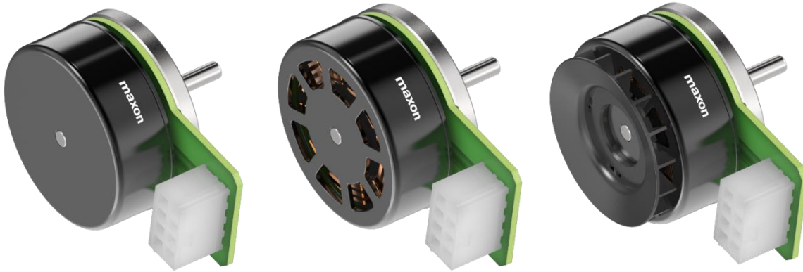
maxon EC 45 flat : Standard version (50/70 watt) – version with open rotor (60/80 watt) and ventilated versions with optimized cooling by a fan (90/120 watt) – from left to right
