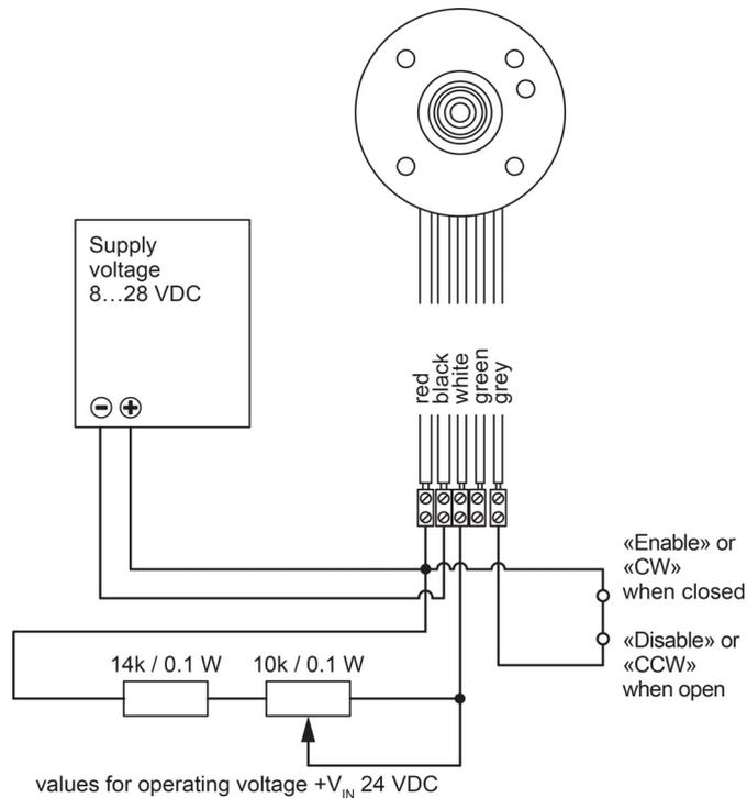
**Figure 6** Set point «Set value speed» via external potentiometer and (depending on version) activation «Enable» or direction preselection «Direction» with potential-free contact
