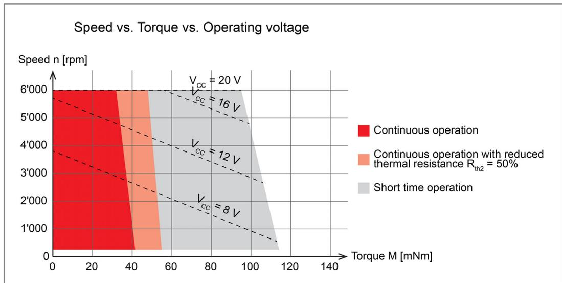
Figure 1 Speed / Torque / Operating voltage diagram
