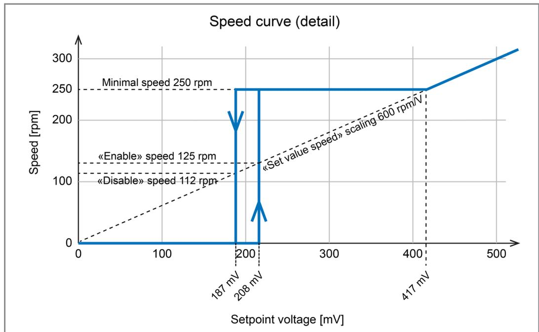
Figure 9 Speed as function of set value voltage – «Enable»
