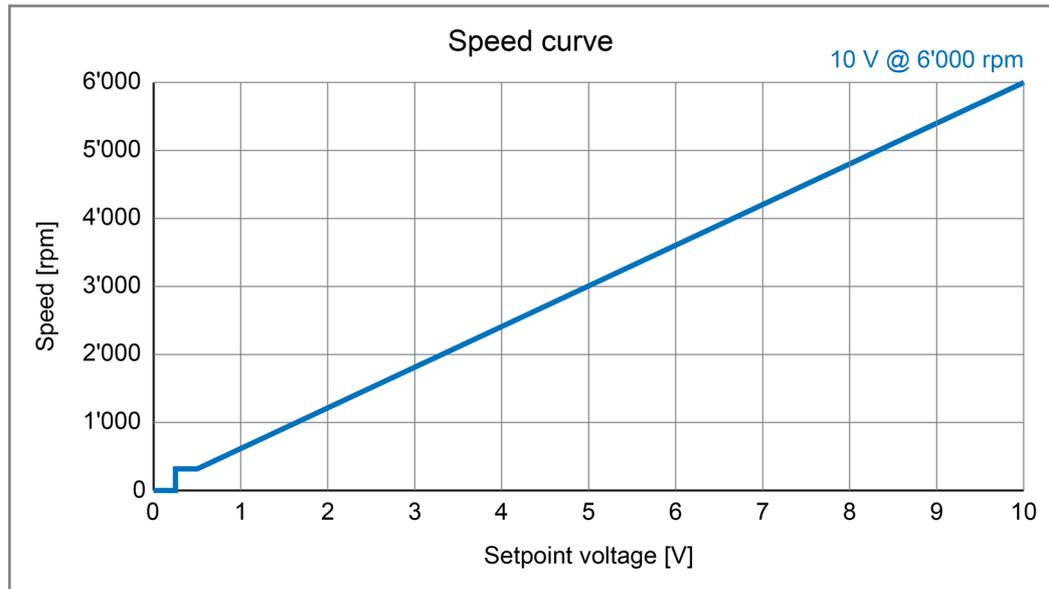
Figure 8 Speed as function of set value voltage
