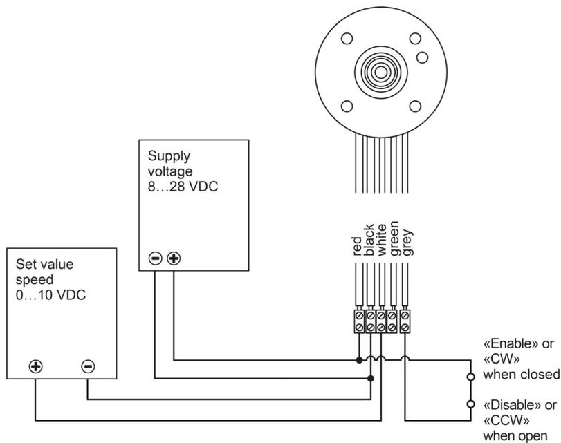
Figure 4 Set point «Set value speed» from external power supply and (depending on version) activation «Enable» or direction preselection «Direction» with potential-free contact
