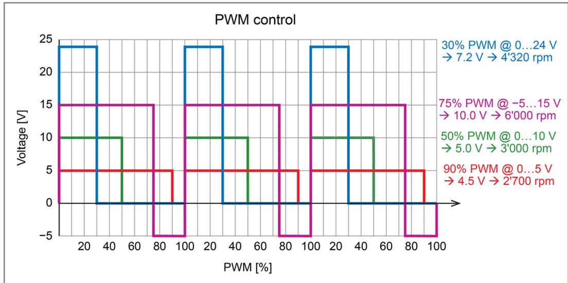
Figure 10      Examples for possible PWM activation for the input «Set value speed»
