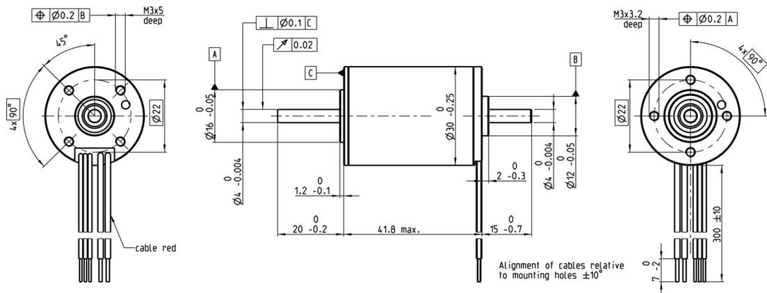
Figure 2 Dimensional drawing [mm]
