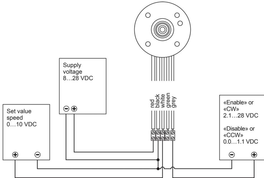
Figure 3 Set point «Set value speed» and (depending on version) activation «Enable» or direction preselection «Direction» from external power supply
