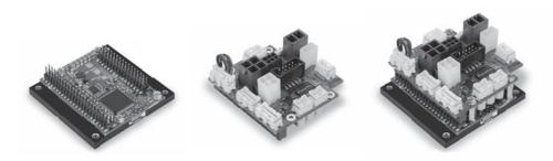
EPOS4 is a modular digital positioning controller. It is suitable for permanent magnet-activated DC motors and brushless, electronically commutated EC motors with incremental or absolute encoders with an operational range of up to 750 W continuous power. The variety of operating modes provides high flexibility: The controllers are suitable for use in a wide range of drive systems in automation and mechatronics.
